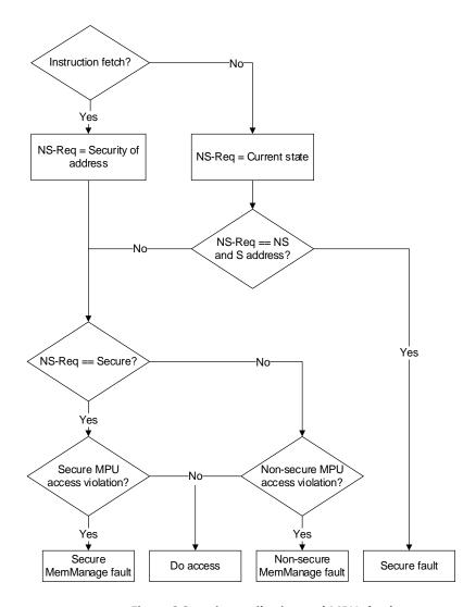
Figure 8 Security attribution and MPU check sequence
