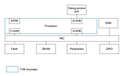
Figure 1 TOE component of a Security IC
